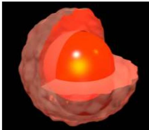
Figure 1.12: Quantum dot sectioned to show the outer shell and the inner core.
