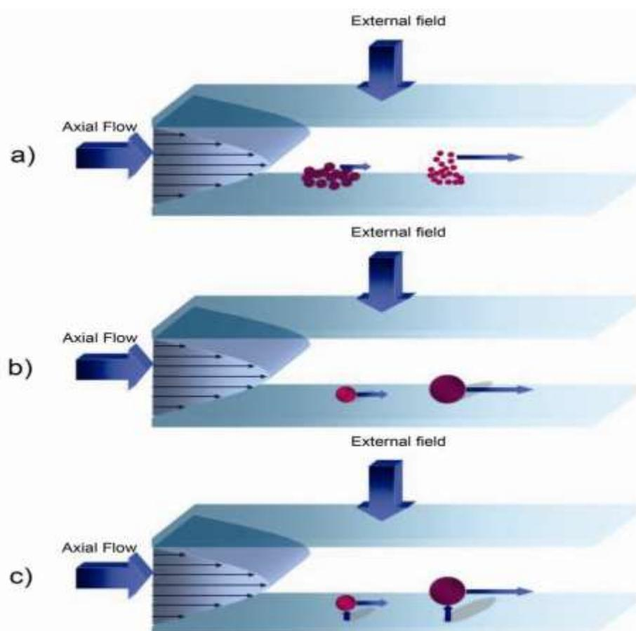
Figure A1.2: Schematic diagram illustrating the typical operation of FFF, showing the mechanism of separation for particles of different size. a) the separation sequence based on particle diffusion coefficients, b) particle separation in steric mode and c) the particle separation in hyperlayer mode (Jamting and Miles, 2013).
