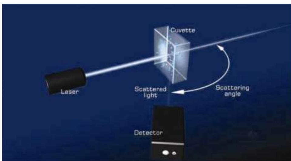
Figure A1.1: Typical DLS configuration: a laser illumination source, a sample under measurement in the cuvette and a detector (Jamting and Miles, 2013).
