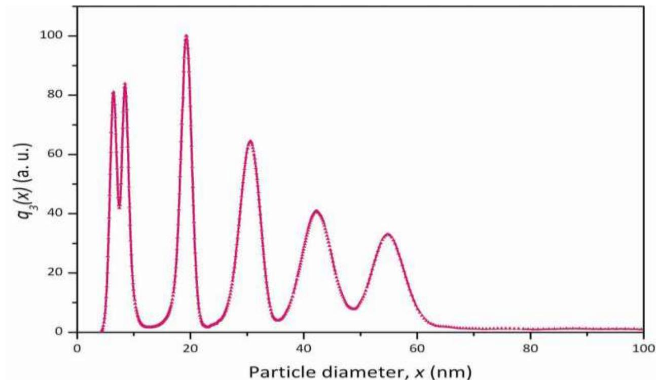
Figure A1.1: Volume-weighted PSD of a 6 modal mix of Au nanoparticles, measured by DCS. The plot illustrates the ability of the technique to clearly separate each of the particle populations in the 6-modal Au suspension (nominal diameters: 5 nm, 10 nm, 20 nm, 30 nm, 40 nm and 50 nm) (Jamting and Miles, 2013).
