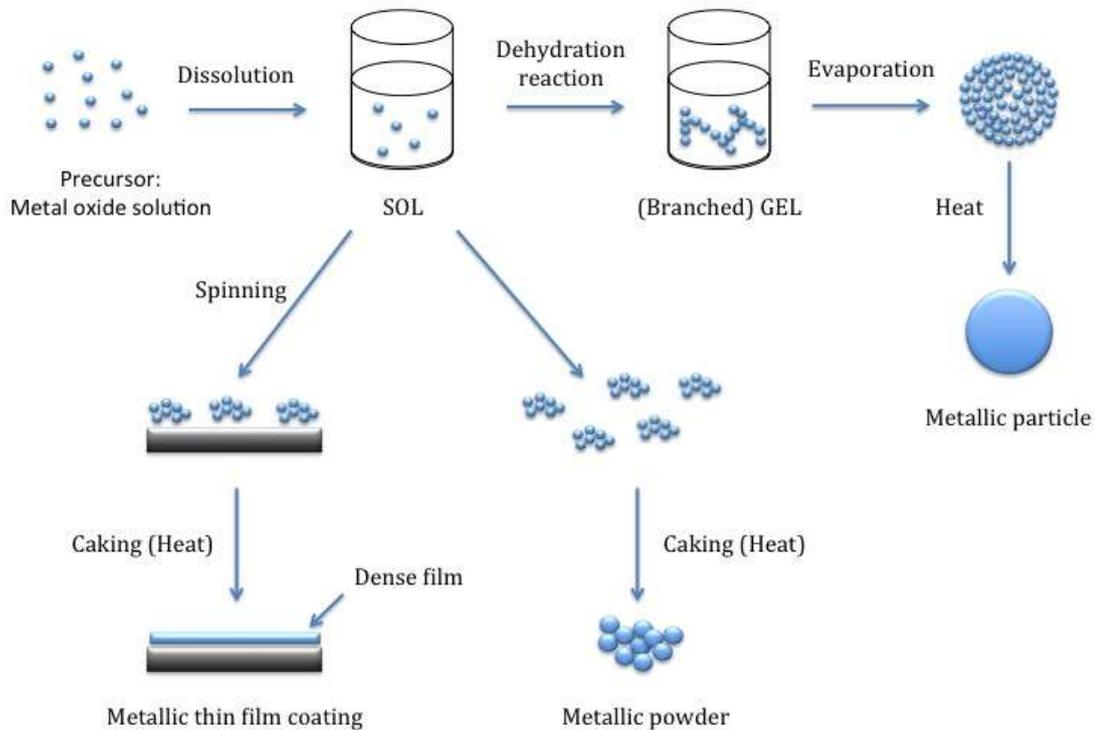
Figure 4.1 The sol-gel process of manufacture (depicted is the fabrication of a metallic thin film coating, metallic powder and metallic particles)
