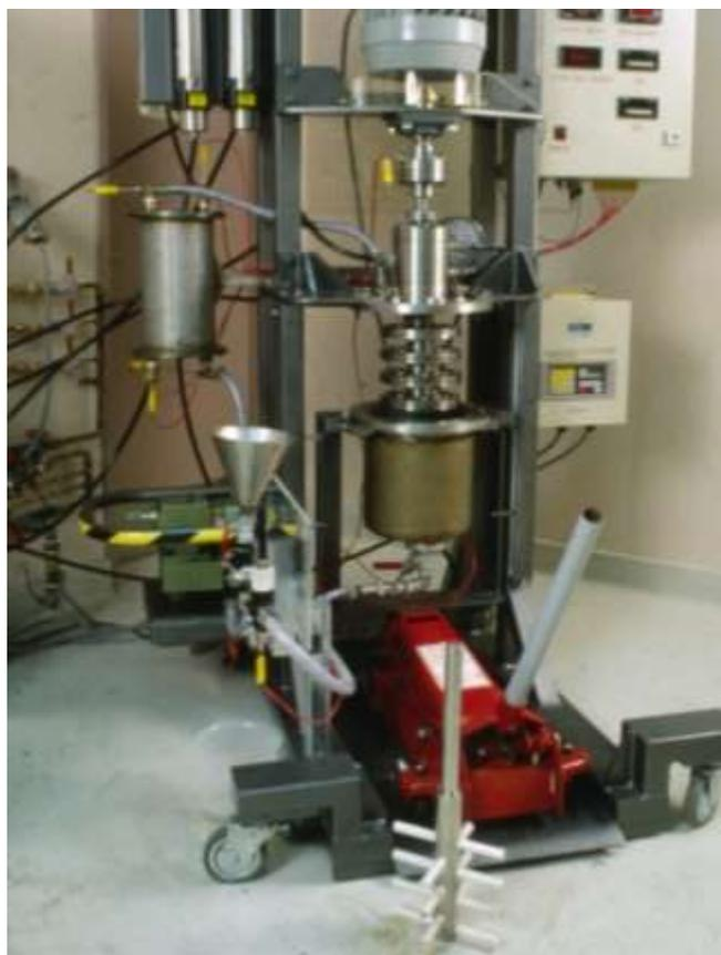
Figure 4.4 Laboratory 'stirred media' mill (with permission T.W. Turney)
