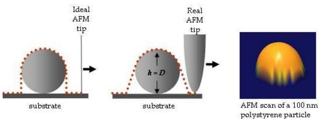
Figure A1.2: A schematic on a substrate being scanned with a) an ideally thin and sharp tip, b) a more realistic AFM tip and c) the result from a 100 nm polystyrene particle scanned with a typical AFM tip (Jamting and Miles, 2013).
