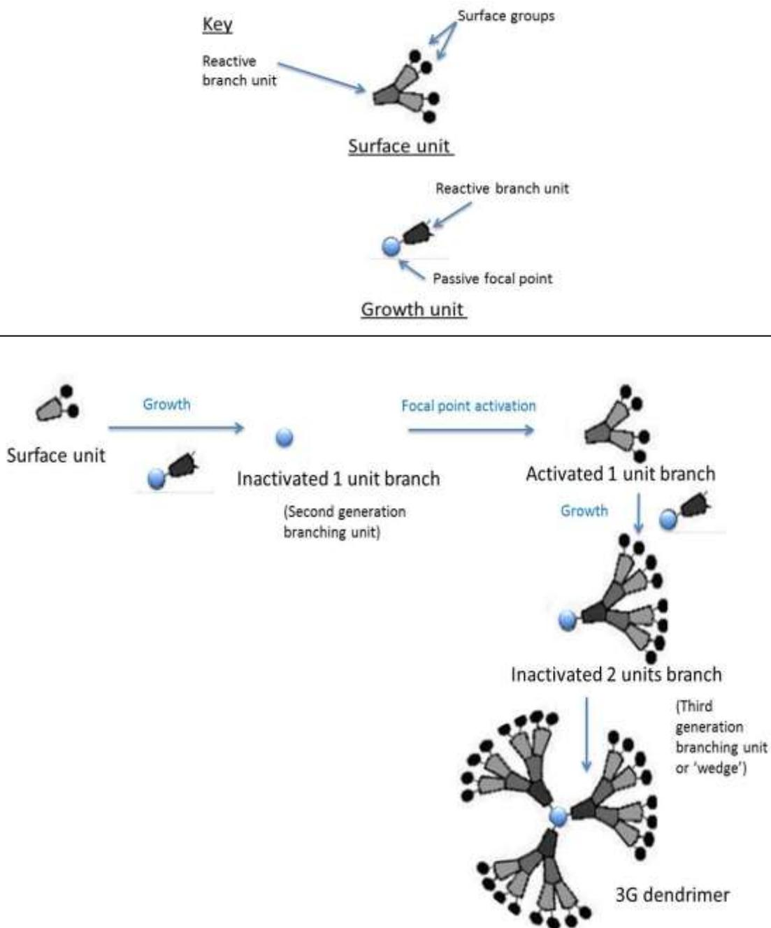
Figure 4.3 The convergent-growth method of dendrimer synthesis.
