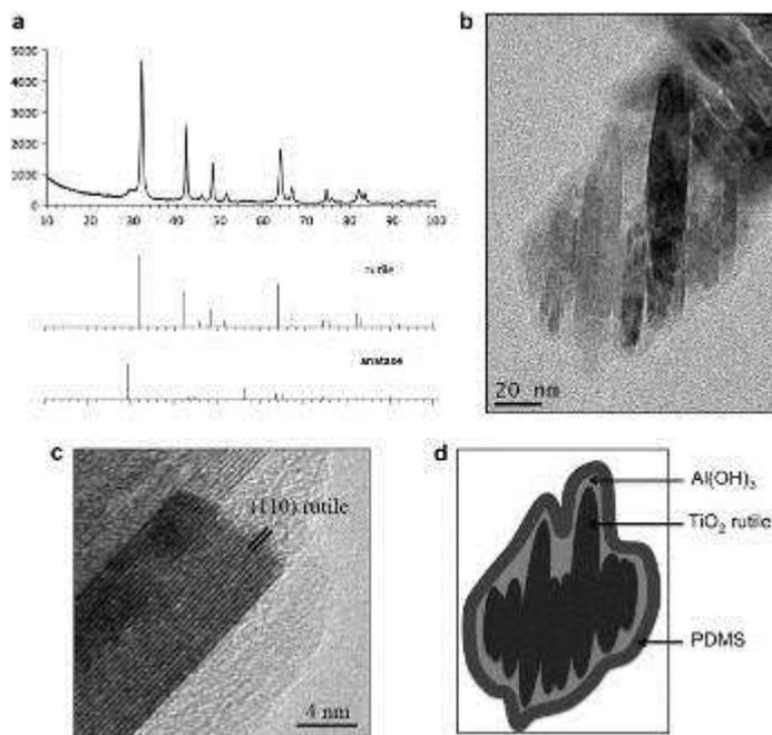
Figure 6.5: An example of a  $\text{TiO}_2$ -based nanocomposite used in sunscreens, characterised by: (a) XRD, (b) TEM, and (c) High Resolution TEM. (d) A schematic view of the formulation highlights the  $\text{TiO}_2$  core, as well as the  $\text{Al}(\text{OH})_3$  and polydimethylsiloxane (PDMS) layers that surround the  $\text{TiO}_2$  nanoparticles. Reproduced with permission from Labille et al, 2010. Copyright 2010 Elsevier.
