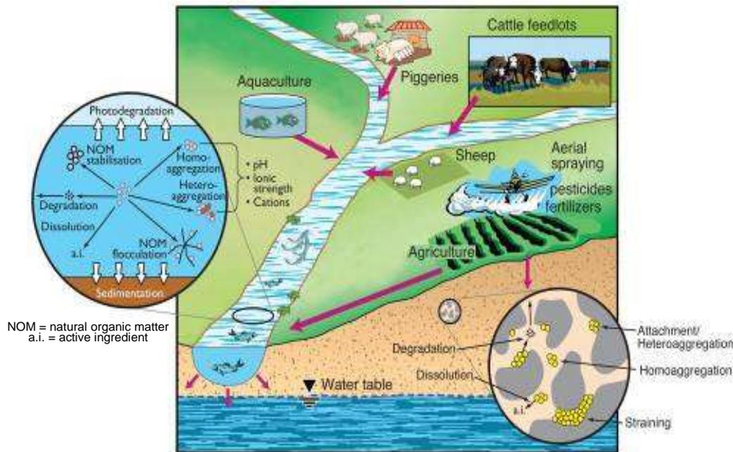
**Figure 6.2:** Potential reactions and fate of nanoscale agricultural and veterinary chemicals in the environment (modified from Batley et al, 2012). With permission from CSIRO, Copyright CSIRO 2013.
