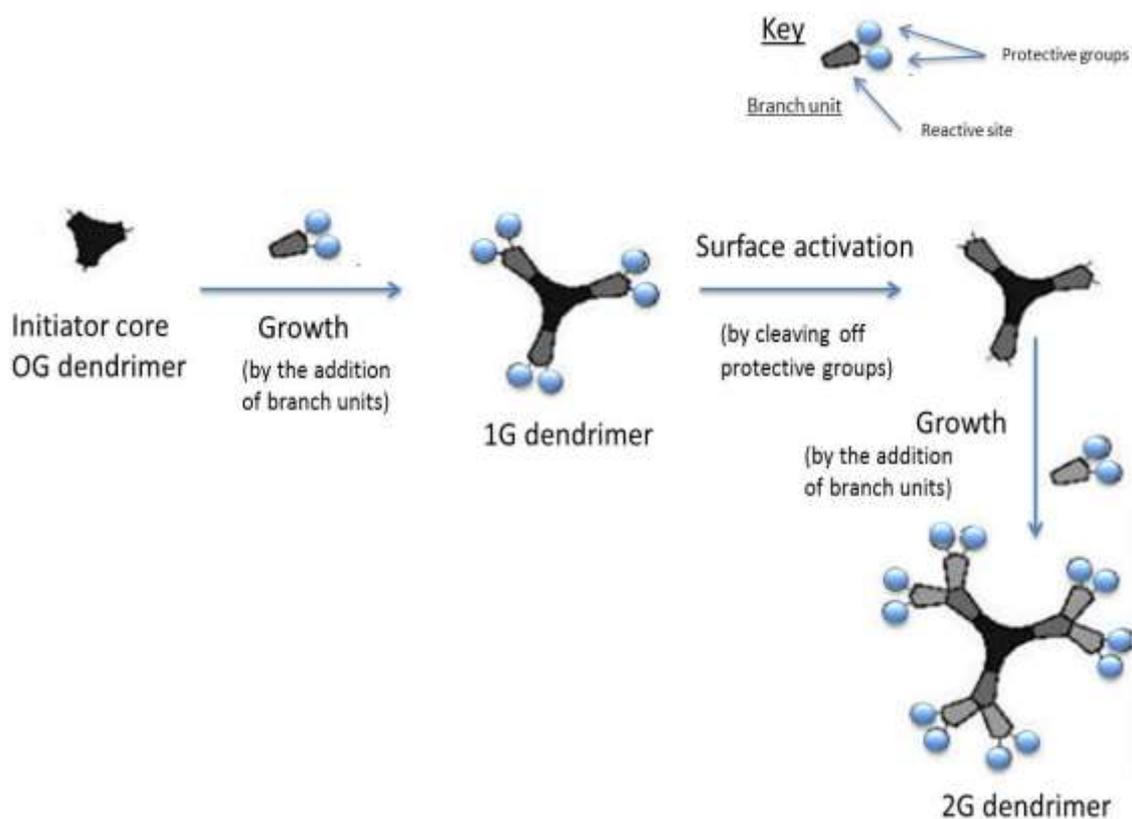
Figure 4.2 The divergent-growth method of dendrimer synthesis.
