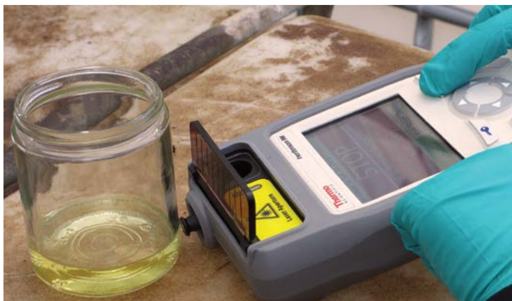
The APVMA's new Raman spectrometer being used by a compliance inspector during a field inspection to identify a chemical product.
